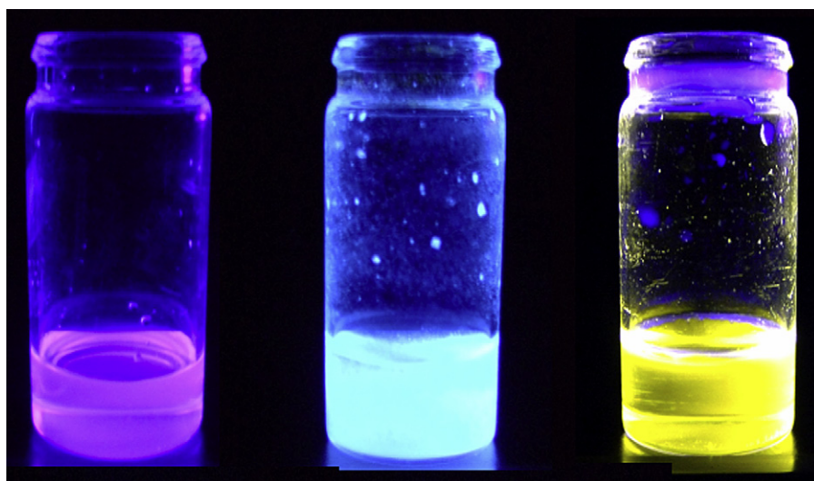
Figure 4. Photographs of NaO-DobPh(5)-ONa when it was irradiated with UV light in \text{CH}_2\text{Cl}_2 (DN=0), THF (DN=20.0), and DMSO (DN=29.8).
